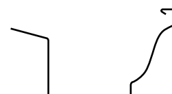
GUTTER WITH BACK FLANGE 1" or 1-1/2" (25.4mm or 38.1mm)
